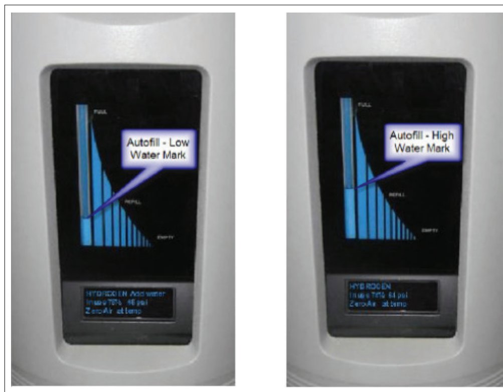
Figure 11 - Typical water levels for an FID Gas Station that is set up with auto water fill
