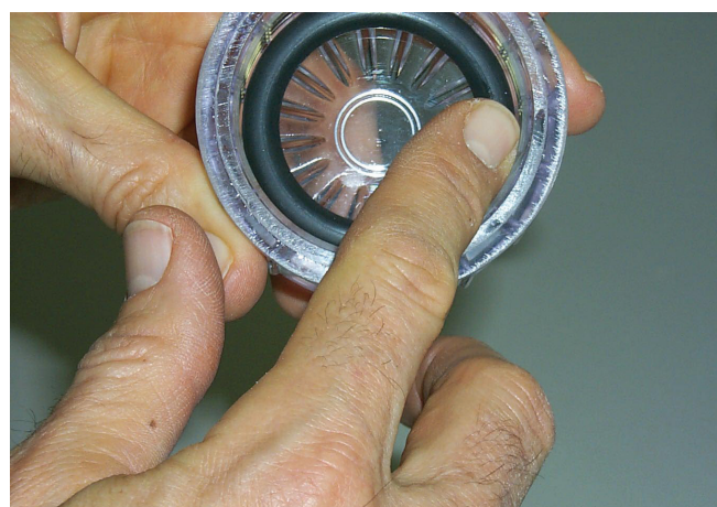
Figure 7 - Make sure the o-ring is centered in the cap before replacing it
