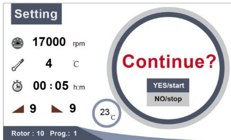
Figure 7-3 Verification of the operation parameters
