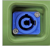
DC Power Connection.
