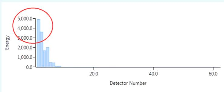
*Figure 10.14 Example of high background signal*
