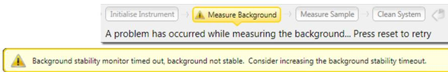
*Figure 10.16 Warning message in the notification panel*
