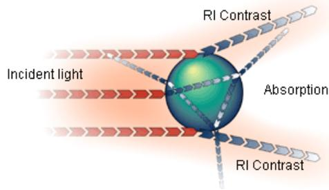
*Figure 9.3 Schematic representation of Mie theory*
