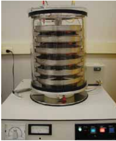
TC60 Tray Cell with Heater Mats and Temperature Controller, on Isolation Valve
