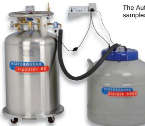
The Autofi II accessory option is particularly useful for the long-term storage of samples within vapour phase environments
