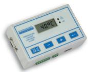
Providing continuous dependable monitoring of the temperature within the refrigerator, the CryoGuard data logger is the ideal choice for users who want to record sample temperature over long periods
