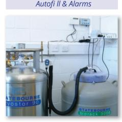
Bio Rack Autofi II and Cryostor option (see next page) connected to Data logger low level alarm and autodialler. Easy withdrawal
