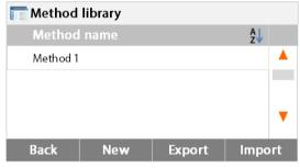
The test library contains 2 methods. All methods which were previously entered can be recalled and the parameters for the recalled method when selected will be repeated.
