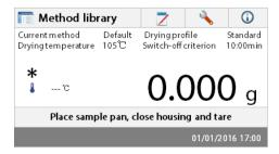
To **switch the Moisture Analyzer on**, press the **On/Off** button. An internal diagnostic test is performed; the display lights and the Home screen appears followed by the initial display.
