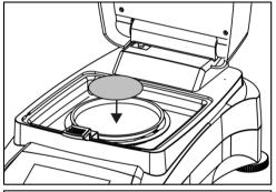
Place the empty sample pan and glass fiber pan in the pan handle. The sample pan must lie flat in the pan handle.
