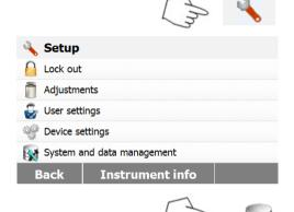
Press Setup button to access Setup menu. Press **Back** to return to Home screen.
