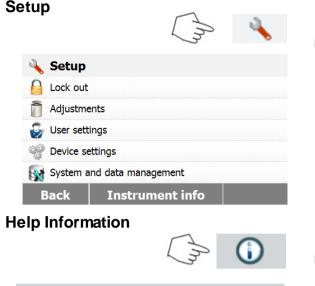
Press the Setup button to access the Setup menu.
