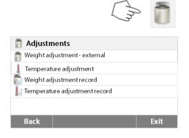
Press the Adjustment button to access adjustment menu.
