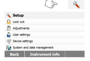
Press Setup button to access the Setup menu.
