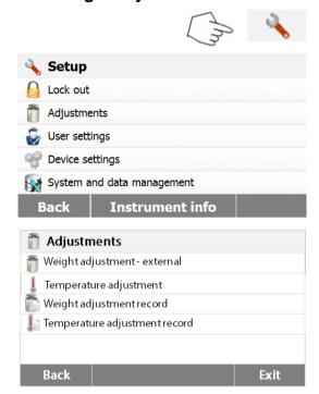
Press Setup button to access the Setup menu.
