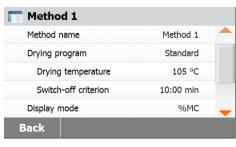
Press the Drying Temperature button to access the temperature setting menu.
