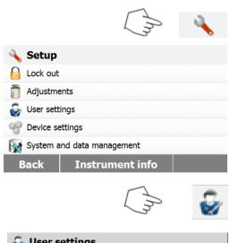
Press Setup button to access the Setup screen.
