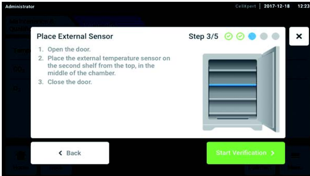
Fig. 10-3: Placement of the external temperature sensor
