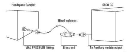
for leak testing
