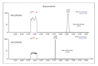
Comparison of UPLC/MS/MS and HPLC/MS/MS for buprenorphine in protein-precipitated human plasma showing improvements in resolution, speed and detection level.
