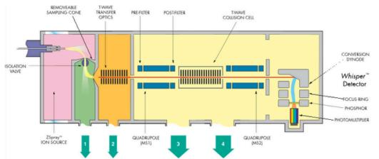
The unique conversion dynode arrangement of the Whisper detector enables stronger signal output and improved limits of detection in negative ion mode, and reduced detector noise levels in both positive and negative ion modes.
