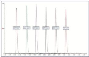
Changing MRM dwell time has no effect on signal intensity even at an acquisition rate of 100 data points per second (5 ms dwell time, 5 ms inter-channel delay).
