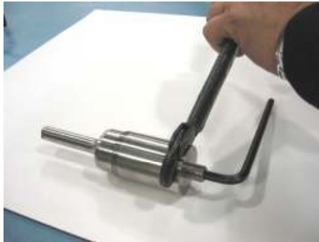
Removing stud from horn
