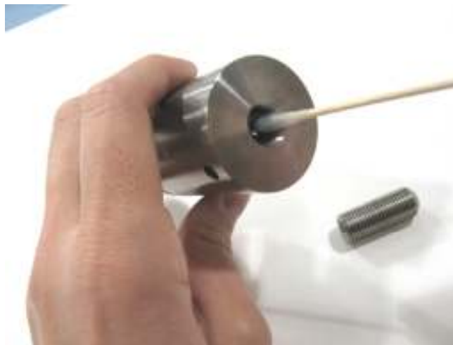
Clean threading inside of horn
