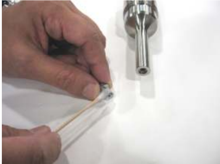
Cleaning replaceable tip threading
