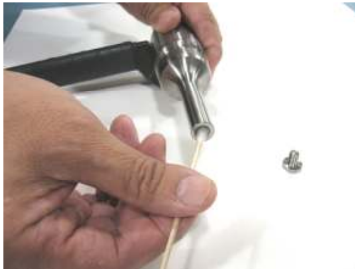
Cleaning horn threading
