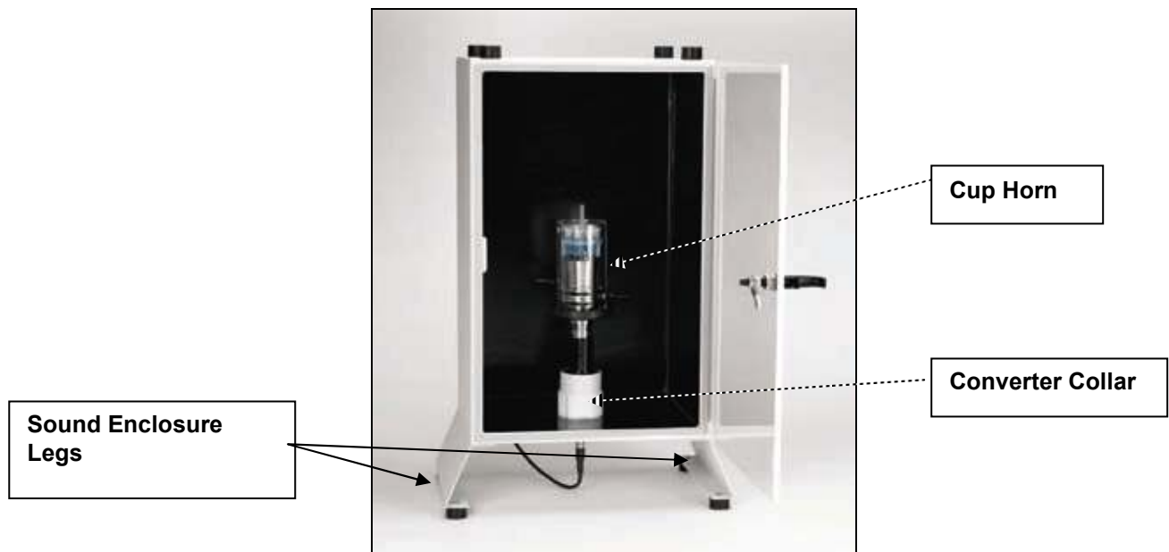
Proper set up of Cup Horn
