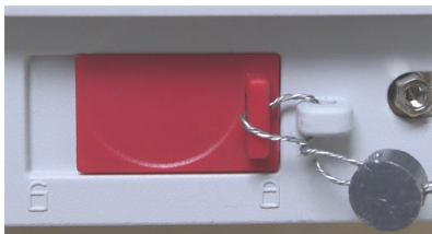
Locked with Wire Seal
