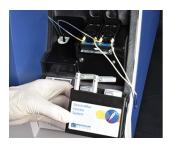
The bottle holder is mounted on two knobs.
