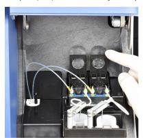
4. Slide the tip into the nozzle, the slots are labeled 1 and 2 for injector 1 and injector 2.
