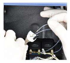
5. Use the black knob to move the nozzle back to the rear of the injector space. Align the nozzle with the opening and press straight down until you feel it snap into place.
