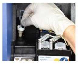
6. Move the injector arm to its original position.
