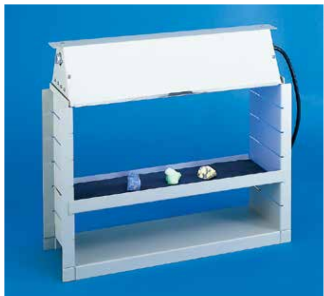
Exposure Stand shelf is adjustable to different levels for exposure of samples.
