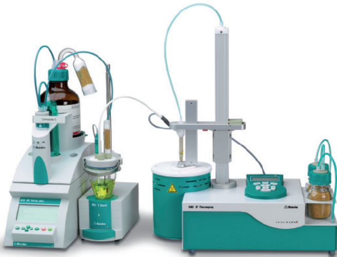
The Karl Fischer oven technique for the easy preparation of difficult samples. The picture shows the 860 KF Thermoprep with manual sample preparation.
