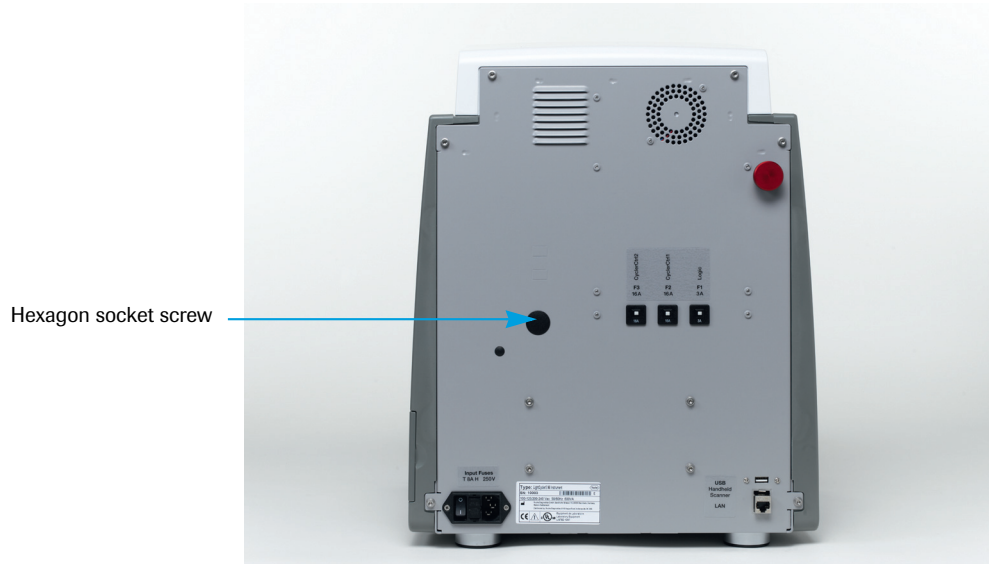
Figure 184: LightCycler® 96 Instrument back view with hexagon socket screw
