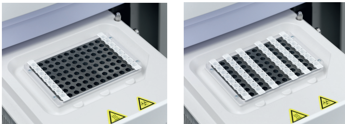
Figure 6: Symmetrical load patterns, examples
