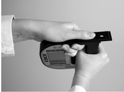
Fig. 12 - 3 Removing the pump lock
