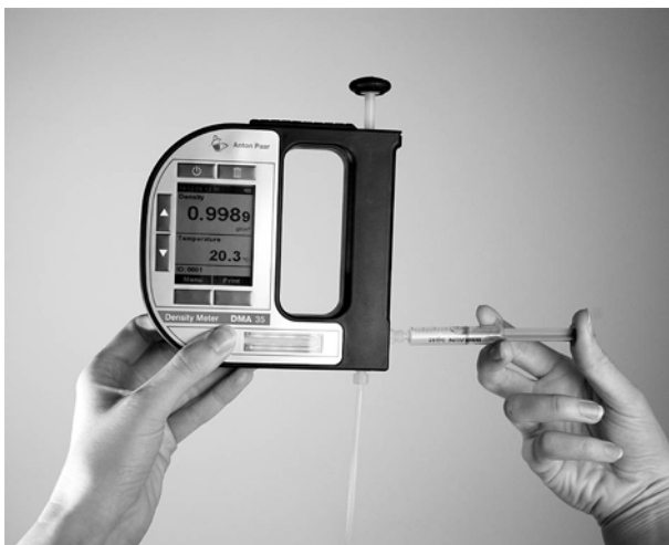
Fig. 10 - 2 Filling sample using the plastic syringe
