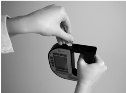
Fig. 12 - 4 Opening the battery cover
