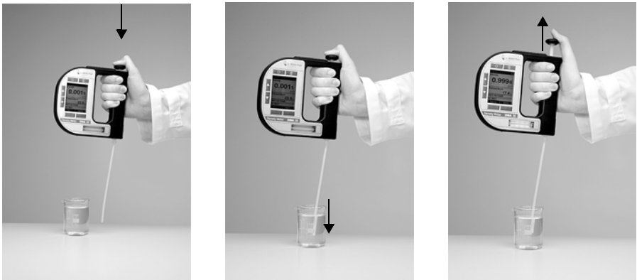
Fig. 10 - 1 Filling sample using the filling tube
