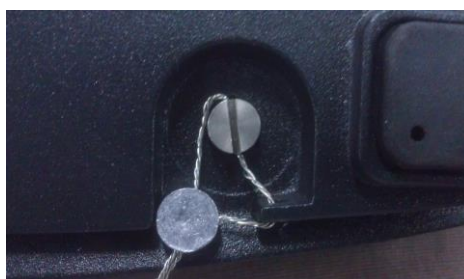
Locked with Wire Seal
