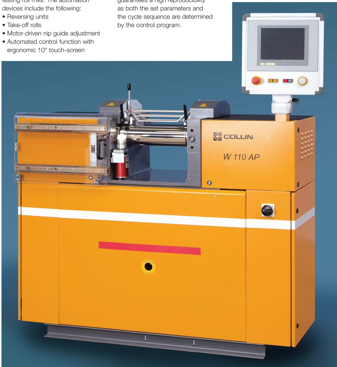
Automated Testing Roll Mill Type W 110 AP with 10" touch-screen control
