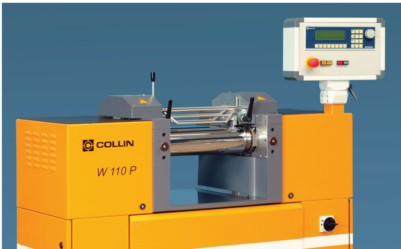
Testing Roll Mill Type W 110 P with SCD-RM sequence control
