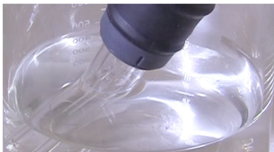
Figure 14. Close up of torch placed in vessel, highlighting acid level relative to the plastic base
