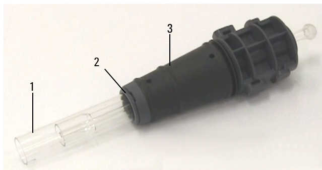
Figure 3. Demountable torch where:
