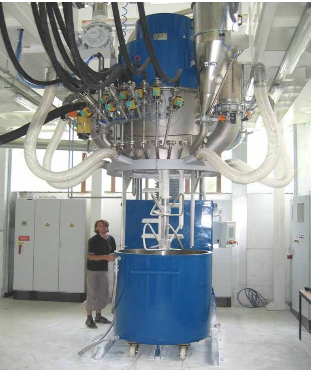
Fully automated, vacuum-tight for sanitary silicone planetary mixer system, model PMH 1000
