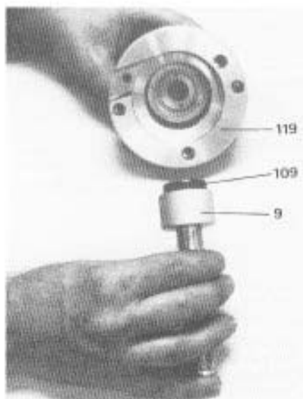
Fitting axial face seal 109
