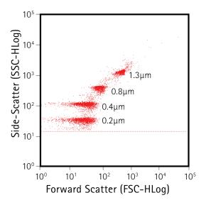
Acquisition of a mixture of beads of known size demonstrates the ability of guava easyCyte $^{\text{m}}$  12 instruments to detect and discriminate particles as small as 0.2  $\mu$ m.
