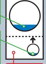
The steam generator stands separate from the autoclave for top loading models.
